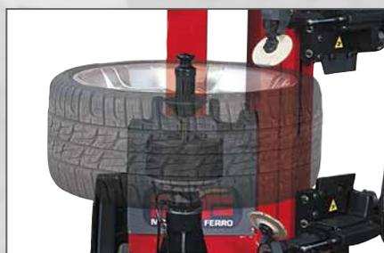
The pedal is used over the wheel preparation and turntable clamping phase, as well as **to release the wheel once the operation has been completed** - this feature is already available with Raptor.
