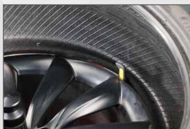
The mounting phase of the second bead is completed by **using the bead breaker disc and the turntable rotation at the same time**, while in case of either lowered tyres or RFT tyres, the Press Mate shall be used to ensure that the tyre remains on the rim channel.
